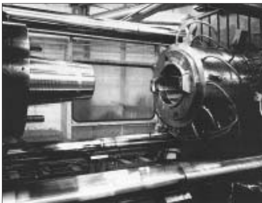
Large mould to produce laundry-baskets. Suitable grade for this moulding tool is Uddeholm Impax Supreme.
