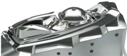
A highly polished mould for production of car headlights. Illustration Graphics, Sweden.
