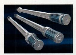
The conventional steel grade was SS 2511, case-hardened, 60 HRC at the surface and softer in the middle. When starting, the enormous torque caused the shaft to twist and fracture. A maximum of three starts could be done before the shafts had to be changed.
