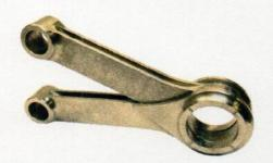
The solution was connecting rods manufactured in **Impax Supreme** with a hardness of 300 HB. Today, the full motor power can be used without deformation of the connecting rods.
