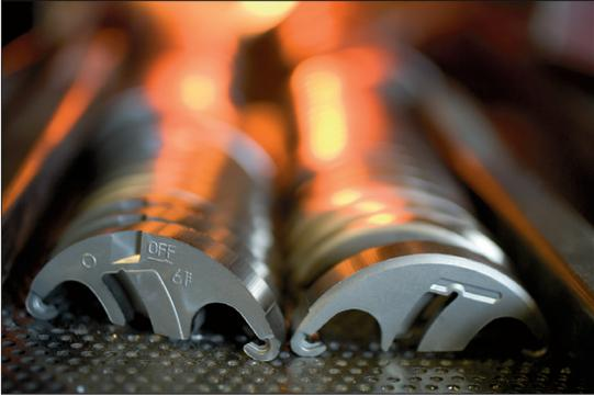
*Sintering of powder compacted parts.*
