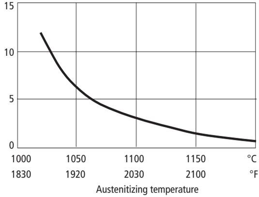
*Total soaking time in a salt bath after pre-heating in two stages at 450°C (840°F) and 850°C (1560°F)*
