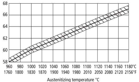
Hardness for different austenitizing temperatures after tempering 3 times for one hour at 560°C (± 1 HRC)
