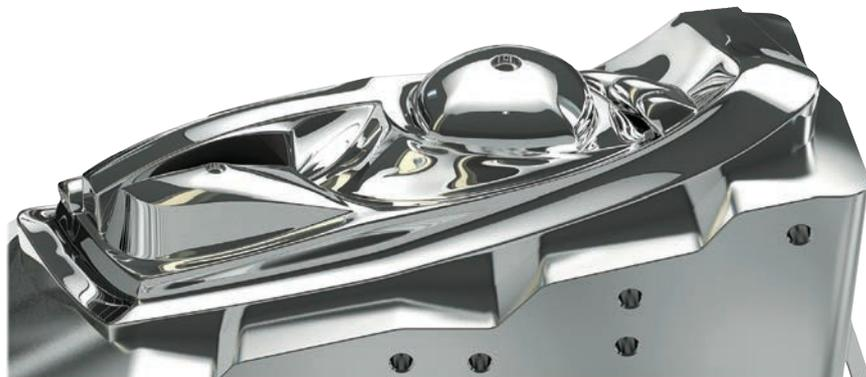
*A high polished mould for production of car headlights.*
